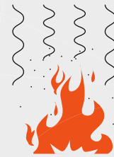
Mist turns into steam, covering the flames and lowering the temperature
